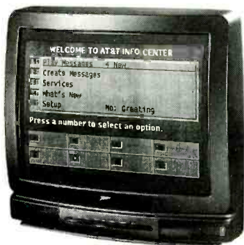
THE AT&T TELEVISION INFORMATION CENTER, available in a set-top box or built-in to a Zenith TV (shown) allows an ordinary TV to be used as a telephone answering machine, for electronic banking, and to supply information services.
